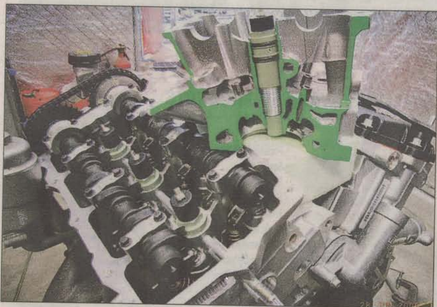
Running time: a GM-H Alloytec, 3.6-litre, V6 petrol engine converted to diesel will be on display at Henty.
